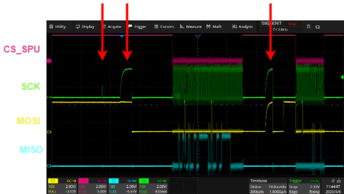
Figure 1. SPI bus traces generated by an Analog Devices MAX78000 host MCU and EVK2. The three red arrows highlight irregular levels in the SCK signal that disrupt the SPU chip on EVK2.
