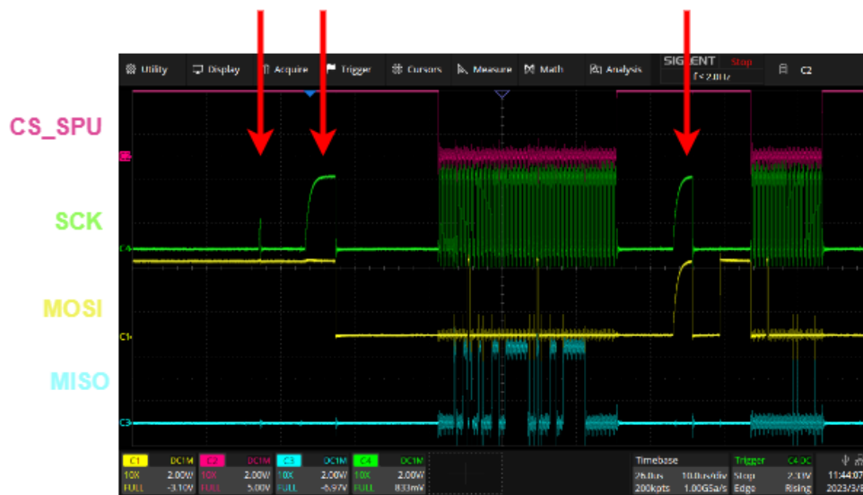
Figure 1. SPI bus traces contaminated by a floating SCK signal when no chips are selected. The three red arrows highlight areas where SPU-001 TC2 is affected.
