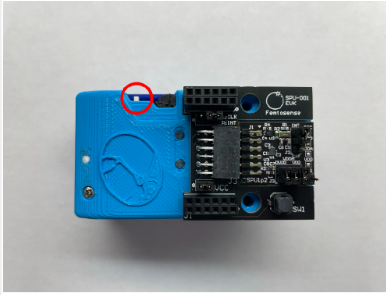
EVK (PCB connector version) with the power switch circled in red.
