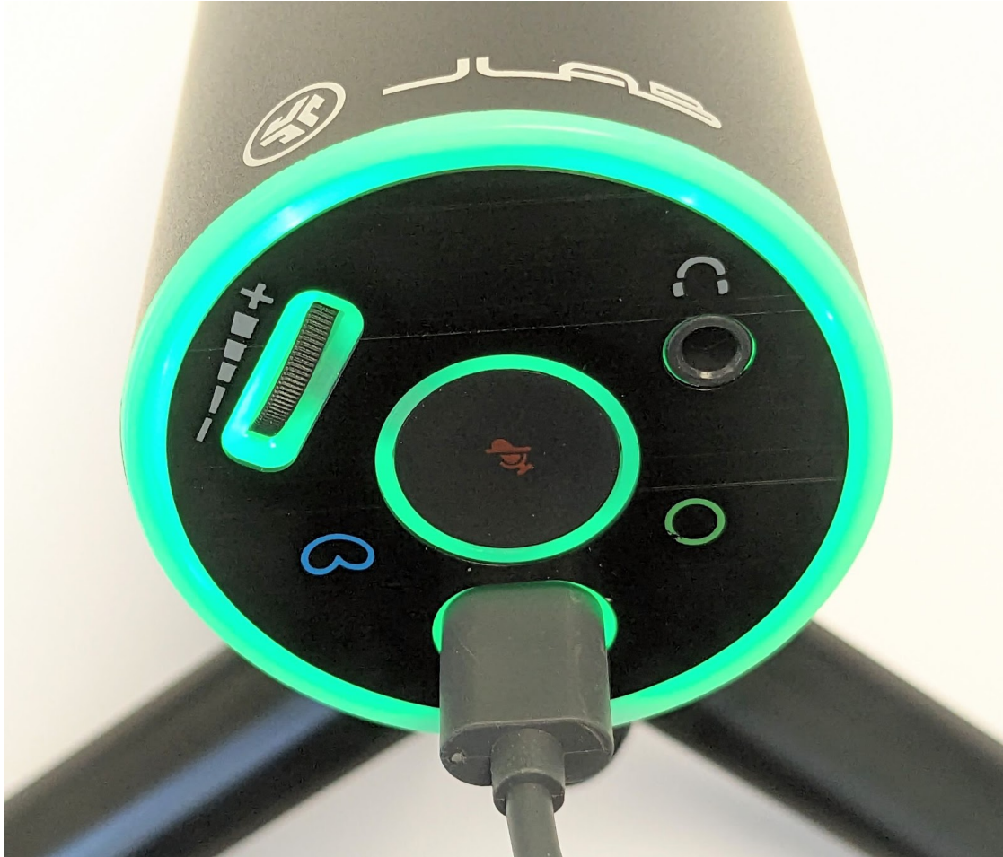
Figure 7: Microphone knob volume control (on the left), and pickup pattern selection light indicator (cardioid in blue and omni in green), select the omni mode by pressing the center button for a few seconds.
