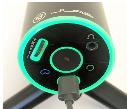
Figure 7: Microphone knob volume control (on the left), and pickup pattern selection indicator (cardioid in blue and omni in green).
