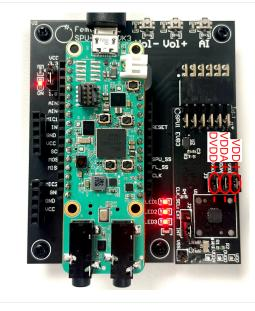
The photo shows the power measurement jumpers for EVK3 (with EVB3)
