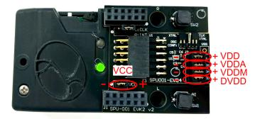
In EVK2+EVB2 shown below, the VDD and VDDM rails are combined together into the single VDD pin:
