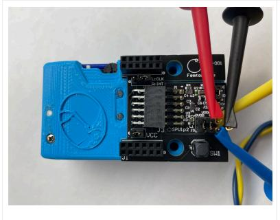
*In the photo, the current and voltage probes measure power on the VDD power rail.*
